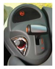
The Auto-Power IV transmission has all powershift and range shift controls on one pivoting T-handle lever.
