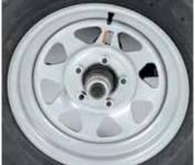
Wheel Bearing Grease Fitting
