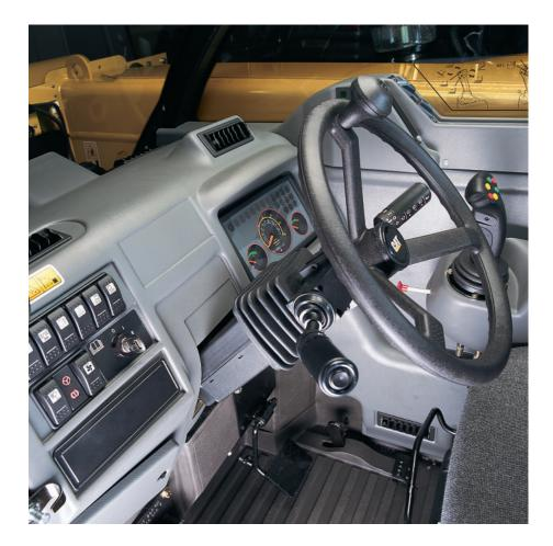
**Enclosed Cab.** The TH215 is equipped with an enclosed cab allowing the operator to work comfortably, with air conditioning available as an option. The cab structure has been designed and certified to provide falling object and rollover protection (FOPS/ROPS).
