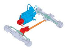
**Hydrostatic Drive.** The TH215 features a high pressure, closed circuit hydrostatic drive to deliver powerful but smooth acceleration while providing continuous torque through the two speed ranges. The low speed band has a maximum travel speed of 8 km/h (5 mph) and the high speed band has a maximum travel speed of 32 km/h (20 mph).
