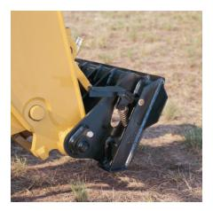
**Manual Coupler.** The TH215 utilizes a manual quick coupler using the same interface as the Caterpillar Skid Steer Loader.
