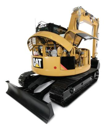
Robust, reliable and easily serviceable are the key attributes of Cat® Mini Hydraulic Excavators. Full steel body work panels and protected front linkage lines are routed neatly out of the way of potential damage above the boom. Easy access to all daily service points are accessed through the rear hood and side cover. A 500 hour engine oil change period lowers operating costs and the Cat S•O•S<sup>SM</sup> points assist easy oil sampling for preventative maintenance checks.
