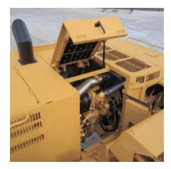
**Emissions.** ACERT Technology is a differentiated technology that reduces emissions at the point of combustion. The technology capitalizes on Caterpillar's proven leadership in three core engine systems: fuel, air and electronics.
