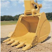
**Ground Engaging Tools.** Caterpillar Ground Engaging Tools (GET) include a variety of side cutters, sidebar protectors, and tip options to match operating conditions.
