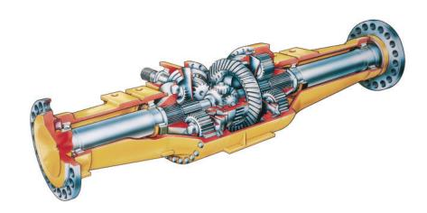
**Front Axle.** Is rigidly mounted to the frame to support the weight of the compactor, internal torque loads and external loads applied during compacting and dozing operations.
