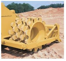
**Outside Mounted S-Blade.** With multiple box section construction including heat treated moldboard and DH-2 steel cutting edges and end bits for long life. The outside mounting is a stronger design because stresses are put on the frame rather than the blade so blade flexing is reduced. It also allows for higher lift and a wider blade can be used than with an inside mounted design.
