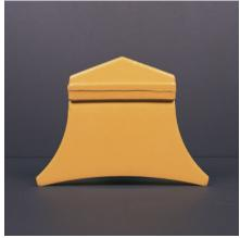
Symmetrical Tamping Wheel Tip Pattern. The modified chevron tamping wheel tip design provides greater ground pressure, more compaction, a smooth ride and excellent traction. Tip height is 190 mm (7.5 in) and width is 168 mm (6.6 in).
