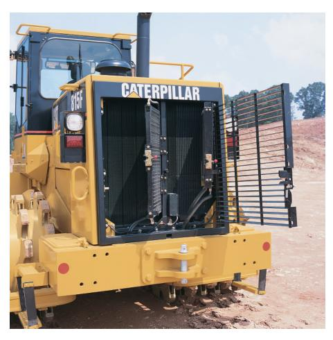
**Battery Box.** Is located in the right side bumper for convenient access to the maintenance-free batteries.
