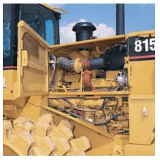
Left Side Service Access. Provides convenient entry to the engine oil filter, grease points (lower), air filter (front), power train oil dipstick (top), coolant sight gauge (top), power train oil fill (below cab), power train oil filter and high speed engine oil fill.
