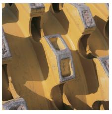
Chevron Tamping Wheel Tip Design. Is used for equal compaction in forward or reverse. Tips are full perimeter and are replaceable. The tip is welded to a base assembly, which is then welded directly to the drum. There are 12 tips per row and 60 tips per wheel for excellent compaction.
