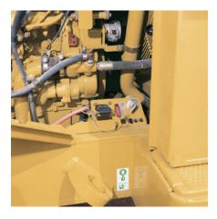
**Engine Shutdown Switch.** Is located inside the left engine enclosure panel for simple access and extended switch life.
