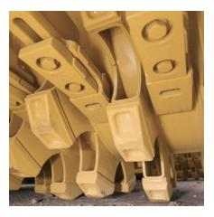
**Adjustable Cleaner Bar Tips.** Are constructed from a ductile iron casting which provides excellent durability and wear life.
