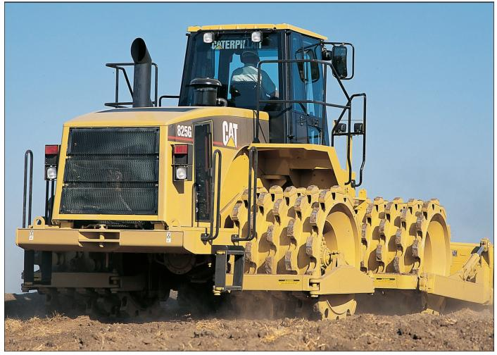
**Modified chevron tamping foot design** provides greater pressure, more compaction, smooth ride, and excellent traction.
