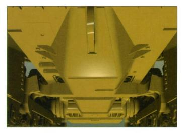
**Crankcase (belly) guards** serve a dual purpose. They help prevent contact damage to vital power train components, and help keep debris out of the power train compartments.
