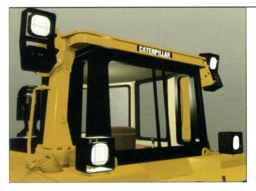
**Rear, tank-mounted lights** are relocated on the ROPS which removes the lights from the concentrated debris environment to help protect them from damage. Combinations vary depending on each model.
