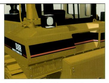
**Hydraulic and fuel tank guard** helps protect implement hydraulic oil tank, battery box and fuel tank.
