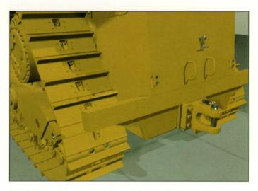
**Rear striker bars** incorporate a rigid drawbar and a housing with large access doors for storage on machines not equipped with rippers. For machines with rippers, striker bars mount on ripper frame.
