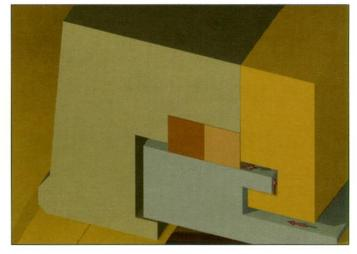
This design offers superior protection to the seal. Debris would have to make four 90 degree turns, penetrate the packing material, and then make two additional 90 degree turns.
