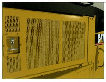
**Engine enclosures** consist of perforated hood and side panels. The enclosures help prevent airborne materials from entering the engine compartment and help reduce radiator plugging which can cause cooling system problems.
