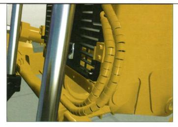
**Tilt cylinder line guards** help protect hydraulic lines from contact damage, while maintaining hose flexibility.
