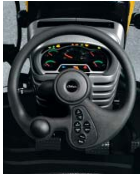
When the transmission is in "Park," the steering is locked out so inadvertent machine movements are avoided.
