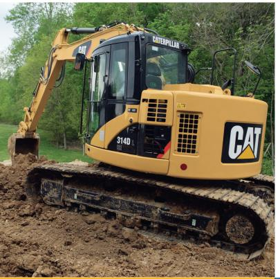
Caterpillar uses advanced engineering and software to analyze all structures, creating a durable, reliable machine for the toughest applications. More than 70 percent of the structural welds are robotic and achieve additional penetration over manual welds. These structural components and undercarriage are the backbone of the machine's durability.
