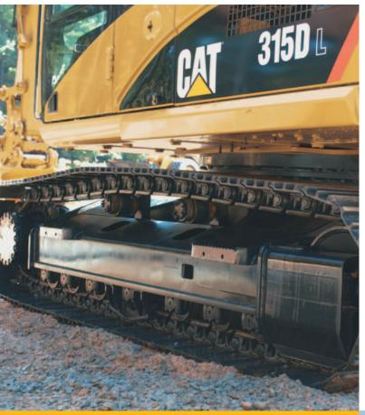
Caterpillar uses advanced engineering and software to analyze all structures, creating a durable, reliable machine for the toughest applications. More than 70 percent of the structural welds are robotic and achieve additional penetration over manual welds. These structural components and undercarriage are the backbone of the machine's durability.
