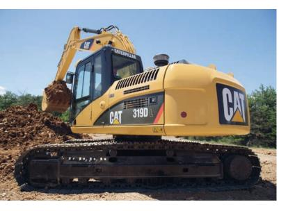
Caterpillar uses advanced engineering and software to analyze all structures, creating a durable, reliable machine for the toughest applications. More than 70 percent of the structural welds are robotic and achieve additional penetration over manual welds. These structural components and undercarriage are the backbone of the machine's durability.
