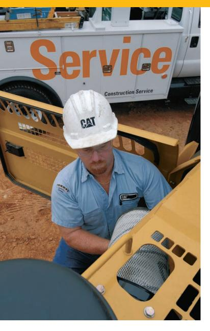
Designed with the service technician in mind, many service locations are at ground level so critical maintenance can be done quickly and efficiently. Longer maintenance intervals reduce cost and increase machine availability.
