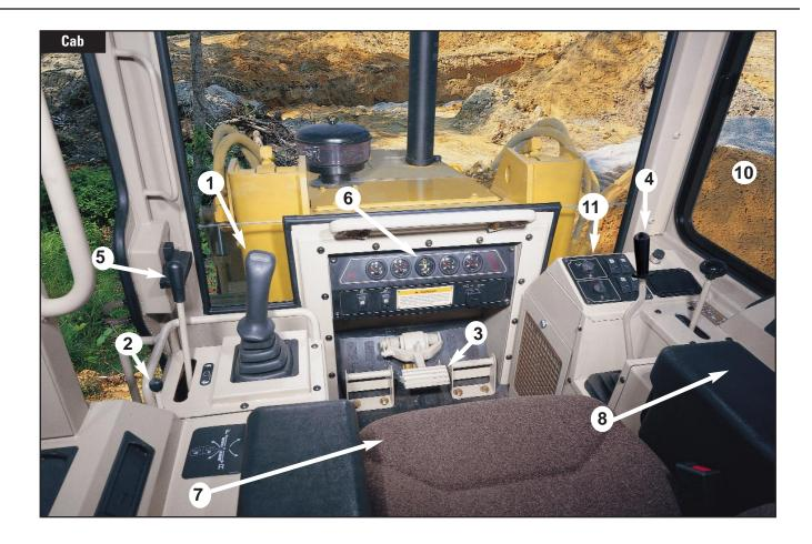
The pressurized cab is sealed to keep dust out and sound to a minimum, resulting in a quiet working environment. Nine adjustable vents keep air circulating and improve the cab's heating, optional air conditioning, and defrost/defog capabilities.
