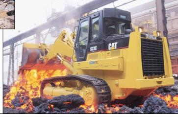
Waste handling/demolition attachments provide added versatility and are designed to make the 973C perform well in landfills, waste handling or demolition applications where the machine spreads, compacts, sorts, shreds and crushes materials.
