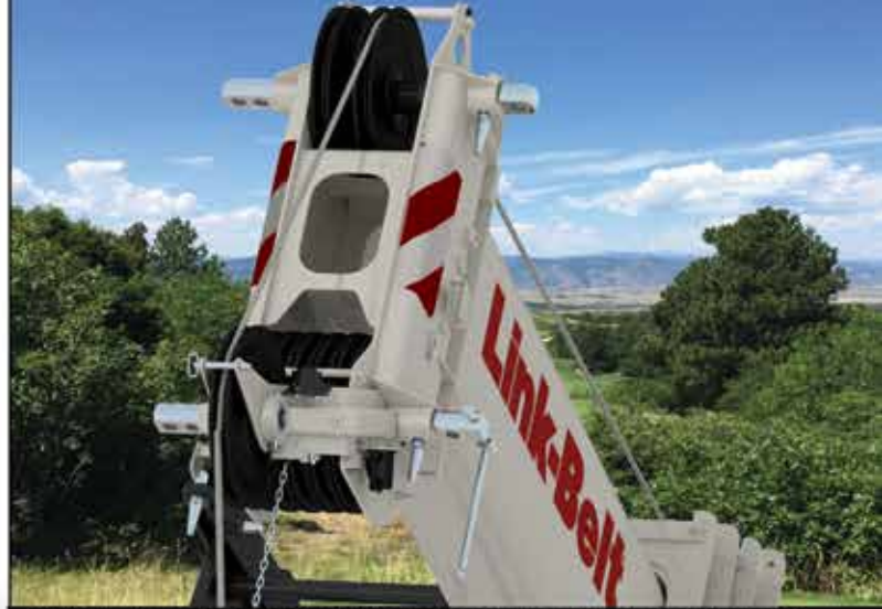
Quick reeve boom head eliminates the need to remove the becket when it becomes necessary to change the reeving
