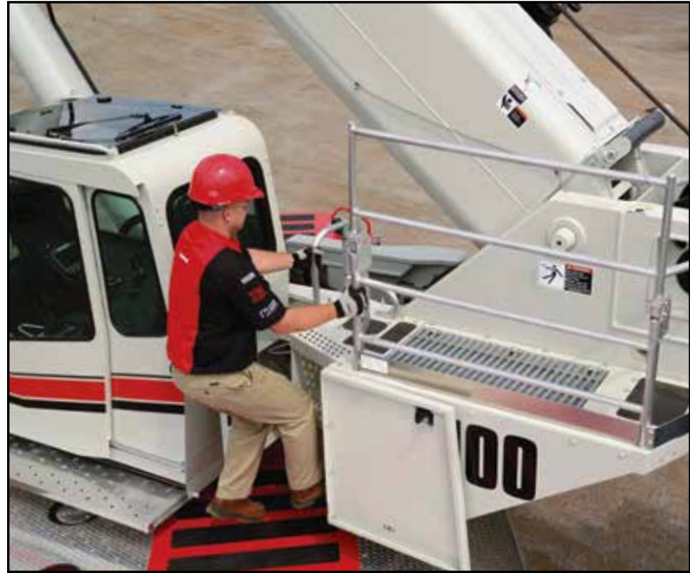
The upper work platform with folding handrails allows for easy inspection and maintenance of the HTC-86100.
