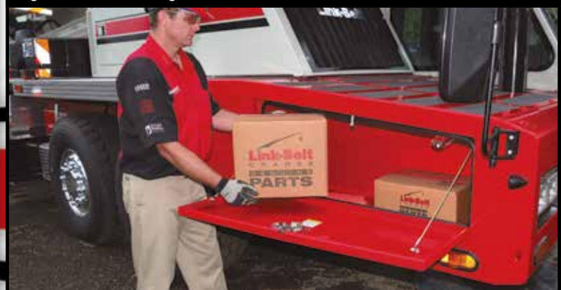
Right side fender storage
