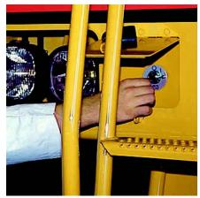
**Ground Level Battery Disconnect Switch.** Facilitates safe, convenient servicing and maintenance.
