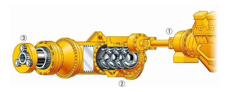
**Transmission.** The Cat seven-speed, power shift transmission, matched with the direct-injection 3412E diesel engine provides constant power over a wide range of operating speeds.
