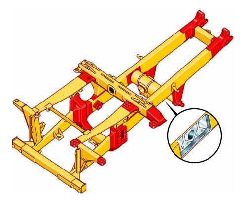
**Box-Section Design.** The 773E frame uses a box-section design, incorporating 20 castings in high stress areas with deep penetrating and continuous wraparound welding. Mild steel, which provides flexibility, durability and resistance to impact loads even in cold climates is used throughout.
