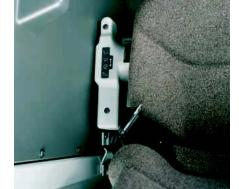
**14) Electrohydraulic Hoist Lever.** Is fingertip actuated and provides low impact body-down snubbing.
