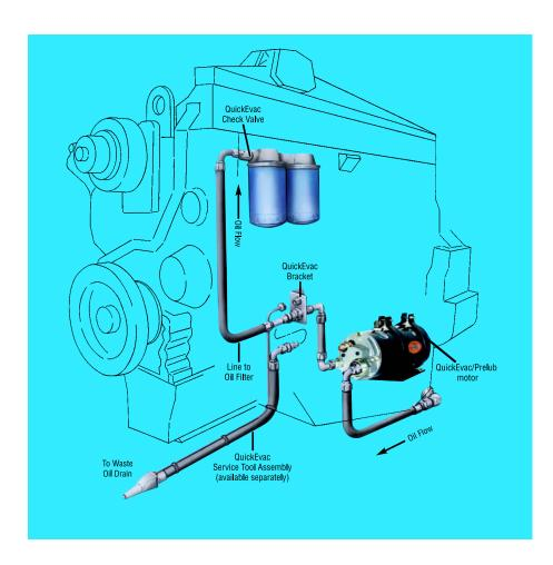
Cat QuickEvac™ System. Is an exclusive Caterpillar on-board engine oil evacuation and prelubrication system.
