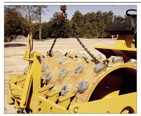
**Two-piece shell kit** features 90 mm (3.5") pad height. Each half of the shell kit weights 453 kg (1,000 lb).
