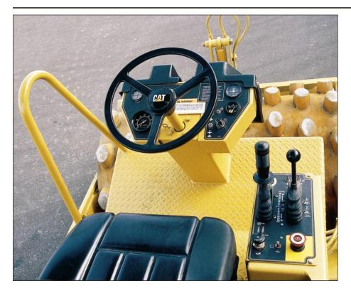
**Single lever control** for propel and vibratory on and off is conveniently located to the right of the operator for simple one-handed operation.
