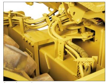
**Secure hose routing** with poly blocks to reduce rubbing and increase service life.
