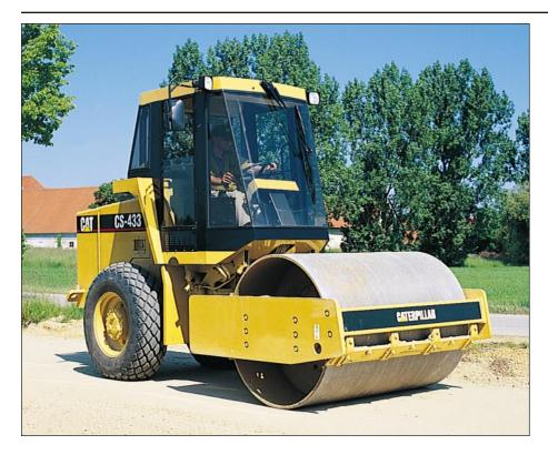
**Sound suppressed cab** isolates operator from noise. 75 dBa at operator's ear.
