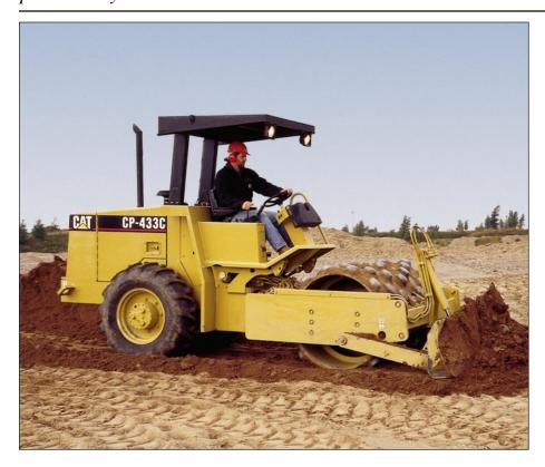
Two-piece reversible and replaceable cutting edges increase edge service life and reduce replacement costs.
